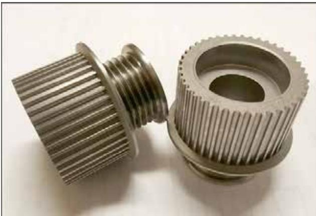
*Fig. 3 This idler pulley is made for a major snow blower manufacturer. The component is made from a machineable grade of FC-0208-50. The splines and precision bores are all pressed in net shape with only the pulley grooves being machined. Bearings are press fitted into the bores and these parts see constant engagement / disengagement during operation. Part strength and freedom from manufacturing defects are all important.*
