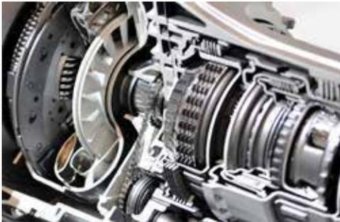
Gears are mechanical hardware that are used to transmit motion, speed, and directional change between axes. Gears are also highly engineered, with complex geometry and require high accuracy which makes them extremely well suited for manufacture in the conventional (mold and sinter) Powder Metallurgy Technology of **ASCO**. Very high production rates with robotic support yield production rates of thousands of parts per hour making for low cost production.
