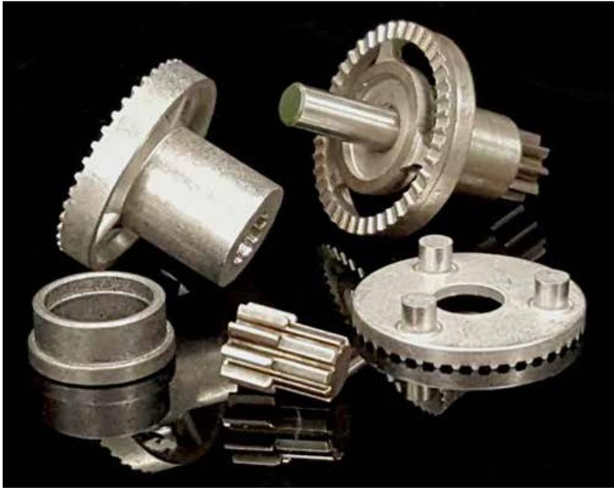
*Fig. 1 Clutch rotor assembly consisting of four parts – an armature, rotor blank, bearing and pinion gear. The assembly operates in a motor drive for automatic sliding minivan doors and opening and closing tailgates. The parts are made to a net shape, except for the rotor which requires a turning operation on the hub. Innovative tooling provides the required part density to satisfy magnetic and strength properties of the rotor*
